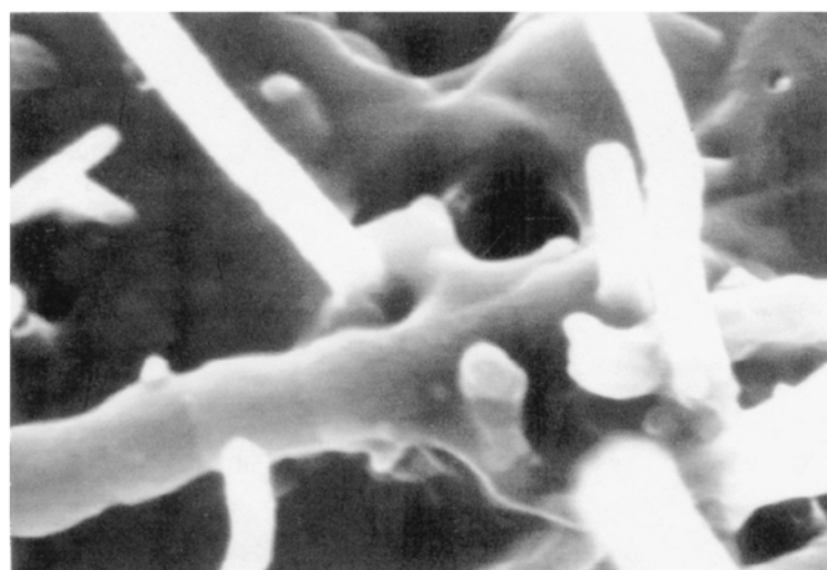
Figure 5 Higher magnification SEM micrographs of the fracture surfaces of polypropylene composites fabricated from Air-Etched and Graphitized fibers.
